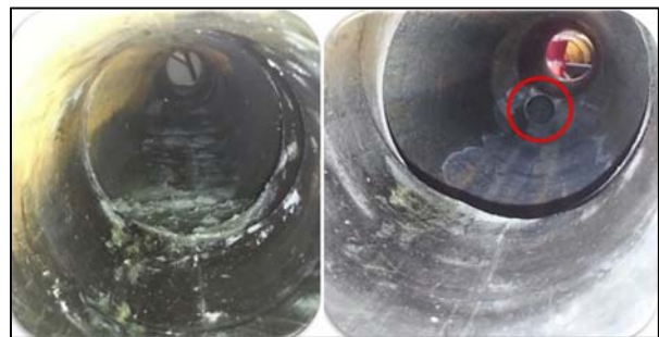
Figure 8. Removal of concrete from a Side Pocket Mandrel (SPM) showing the concrete on the left, and the cleaned SPM with the opening visible on the right.
