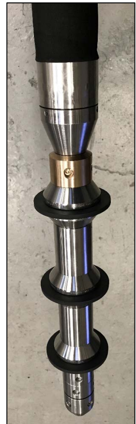
Figure 10. Fluid Hold-Up Tool (FHUT) attached to the bottom of the WASP® tool
