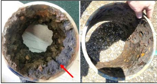
Figure 9. Removal of iron carbonate scale ( \text{FeCO}_3 ) from 9-5/8" casing using EHP. The photo on the left shows the scale, including where an attempt was made to remove scale with a hammer and screwdriver (red arrow). The photo on the right shows the piece of casing after only 120 pulses.
