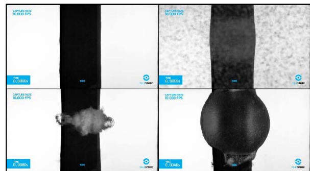
Figure 6. Clockwise from top-left, high-speed photos of an EHP tool pulsing, showing the creation and subsequent collapse of a cavitation bubble.
